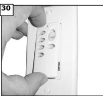
Attach cover of remote by placing over buttons and snaping into place.
